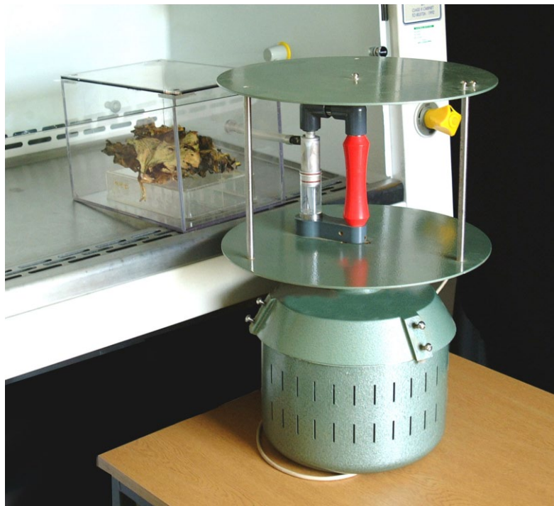
Plate 1. Collection of airborne spora in to an eppendorf vessel employing a Burkard cyclone sampler.
